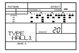
2 Set the desired type by rotating the Jog Dial or by using the +1 and -1 buttons.
