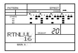
2 Set the return level by rotating the Jog Dial or by using the +1 and -1 buttons.
