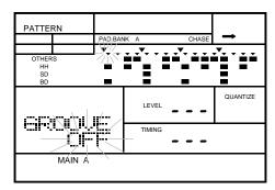
Select the groove by rotating the Jog Dial or using the +1 and -1 buttons.
