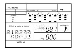
Change the level by rotating the Jog Dial or by using the +1 and -1 buttons.
