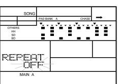
Change the value from "OFF" to "ON" by rotating the Jog Dial or using the +1 and -1 buttons.
