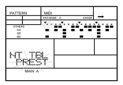
Select a table by rotating the Jog Dial or by using the +1 and -1 buttons.
