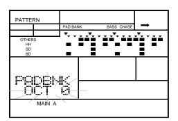
Select an octave range by rotating the Jog Dial or by using the +1 and -1 buttons.
