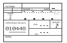
Complete the second measure by repeating the above procedure. Once the RY20 has looped back to the beginning of the first measure, you can record the snare drum, hi-hat, or other parts.
