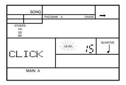
2 Set the volume by rotating the Jog Dial or using the +1 and -1 buttons.
