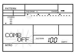
The initial track selected is the "BD" - bass drum - track. Notice the track " • " indicator is lit. You can change tracks by pressing the appropriate Track Select/Mute button.
