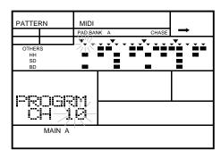
Select a receive channel by rotating the Jog Dial or by using the +1 and -1 buttons.
