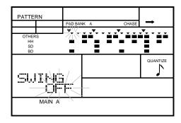
**2** Set the swing by rotating the Jog Dial or using the +1 and -1 buttons.
