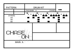
The chase mode is either "ON" (the default) or "OFF". Change the mode by rotating the Jog Dial or by using the +1 and -1 buttons.
