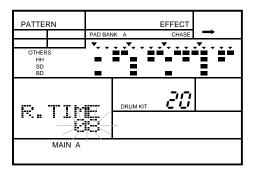
2 Set the reverb time by rotating the Jog Dial or by using the +1 and -1 buttons. The range is from "00" to "31".
