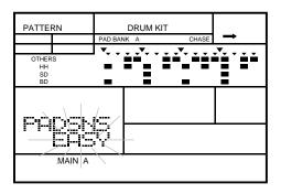
2 Select the pad sensitivity by rotating the Jog Dial or by using the +1 and -1 buttons.
