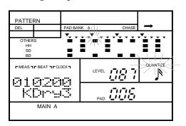
Press the appropriate drum pad, for example, the 6 - BD pad. The note indicator for the event turns off.
