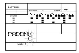
The RY20 has five pad banks labeled "A" to "E". Each pad bank contains 12 drum pads. This indicates that a drum kit can accommodate 60 drum or percussion voices (pad numbers "00" to "59"). See page 83 for more information.
