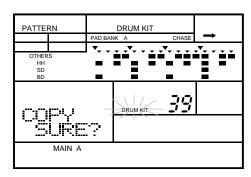
Select a drum kit from "20" to "39" to copy to by rotating the Jog Dial or by using the +1 and -1 buttons.
