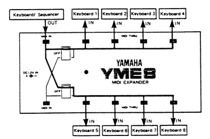
EXAMPLE 2) With this set up, the keyboard/sequencer connected to MIDI IN 1 controls the keyboards connected to MIDI THRU 1 to 4. And, the keyboard/sequencer connected to MIDI IN 2 controls the keyboards connected to MIDI THRU 5 to 8.
