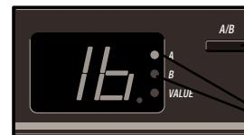
The setting of A/B determines whether the A or B versions of presets and registers will be loaded.
