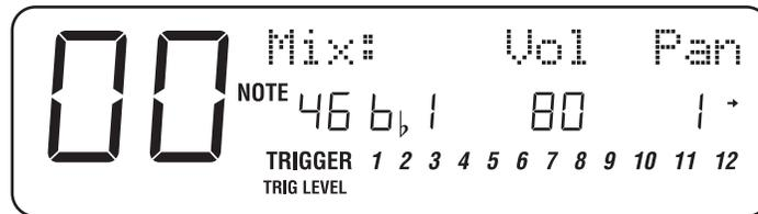
To change the Volume, use the [◀] and [▶] buttons to place the cursor under the VOL value and turn the [VALUE] knob. Values are variable from 00 to 99.
