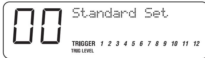
To select a particular Drum Set, turn the [VALUE] knob. The range is from 00 to 20.
