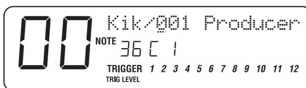
In the upper section of the display there will appear two parameters: Voice Family and Voice Number (a slash / appears between them). The above example shows Note #36 (C 1) is selected, and its assigned Voice is the first sound (001) in the Kick (KIK) Family. Note that the Voice Number (001) is underlined, indicating that it is selected for editing (using the [VALUE] knob).
