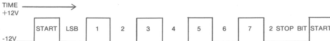
Because RS-232C is an inverting data format, the data shown above would be 01010101 binary or 55 hexadecimal.
