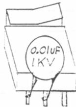
Capacitor leads must be wrapped 360 degrees around switch leads and then soldered..
