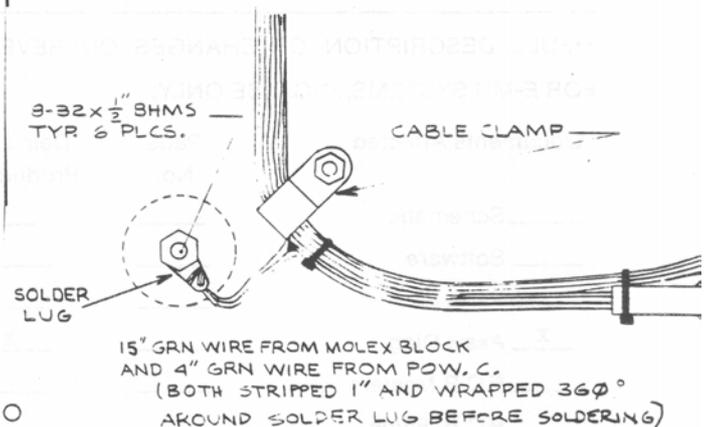
2. Then wrap wires 360 degrees around solder lug before soldering.
