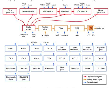
The audio signal flow is represented in red (digital path) and then in orange (analog path):
