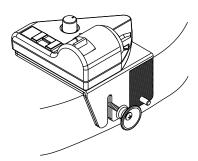
4. Tighten the Holder "A" and "B" with Wing Nut, Spring Washer, Washer.
