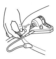
Before playing, be sure to wrap the cable around the guitar strap near the strap hook.
