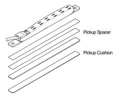
\* The pickup spacers and the pickup cushion are attached to the guitar with double-sided tape which will become thinner by 0.1 mm (0.004") when the backing is removed. Therefore, when using several pickup spacers, you must set the height slightly higher to compensate.
