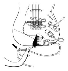
2. Connect the large plug of the supplied (short) guitar cord to the output jack on the guitar, and the smaller plug to the Normal Guitar Input Jack on the Controller.
