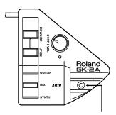
Put the screw (flat-head) through this hole.
