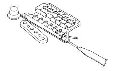
(3) Carefully remove the double–sided tape from the bottom of the Pickup as shown:
