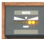
This display shows you all adjustable values for every parameter of the chosen preset . Turn a knob long enough so the LED (PRESET) in the middle blinks. If the changed value is smaller than the one in the Preset, then one of the three LEDs (left) will light up. Should the value be greater, then one the first LEDs (right) will light up. In this respect, you can easily make out the Preset's value.
