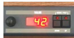
Choose between the monophonic / polyphonic mode by pressing DOWN and UP button at the same time (MONO/POLY). The display will show "of" for monophonic and "on" for polyphonic mode.
