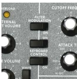
Here you can activate additional Filter-Modulation. The source will be the signal defined within the Modulation-Mix section. This can be Oscillator 3, Noise or a mix of both. Intensity can be adjusted by using the Modulation-Wheel and its additional parameters.
