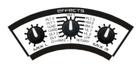
The Revolution provides 16 preset stereo 24 bit DSP effects for processing both internal and external sounds. Although the internal sound section of the Revolution is mono, these stereo effects can be used to widen the stereo field of the sound as well as provide more depth.
