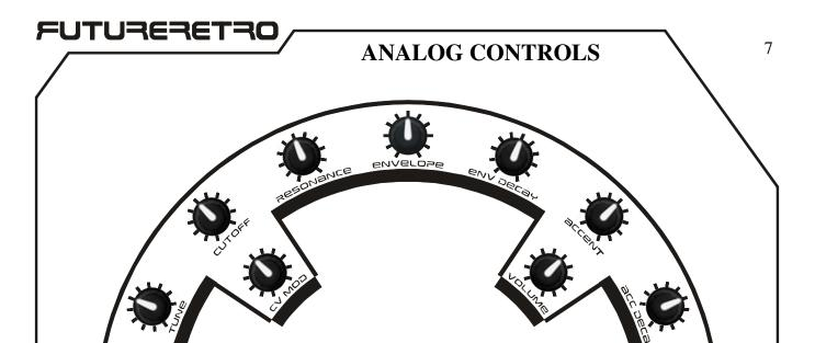
**TUNE** This is a fine tune control for the pitch of the oscillator. It has approximately a +/- 1 semitone range. When this control is in the mid-position, the oscillator should generate the correct pitch programmed into the sequencer. Use this control to fine tune the Revolution with other equipment. If larger changes in frequency are required, you can transpose the patterns within the sequencer.
