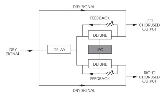
**Mono Flange.** First used in the 1960s, "Flanging" was achieved by the use of two tape recorders that would record and play back the same program in synchronization. By alternately slowing down one tape machine, and then the other, different phase cancellations would occur. Since the slowing down of the tape machines was done by hand pressure against the flanges of the tape supply reels, the term "Flanging" came into being.
