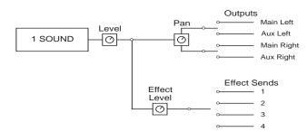
The Effect Patch's *Configuration* determines the arrangement of effect functions of each effect send. Imagine a Configuration as an arrangement of multiple effects processors patched together at the end of each effect send.
