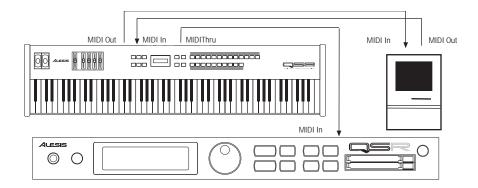
If you are driving other MIDI gear (such as an expander module or MIDI-responsive signal processor), you'll usually drive these from the sequencer if it has additional MIDI outputs. However, you can also use the QSR's [MIDI THRU] connector to drive other modules since the Thru carries a replica of what appears at the QSR's [MIDI IN], which is the same as the sequencer's MIDI OUT.
