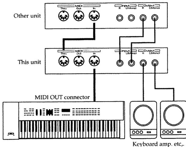
If you connect the output jacks on another sound module to the unit's Input jacks, you can listen to the sounds output from the two sound modules without using a mixer.
