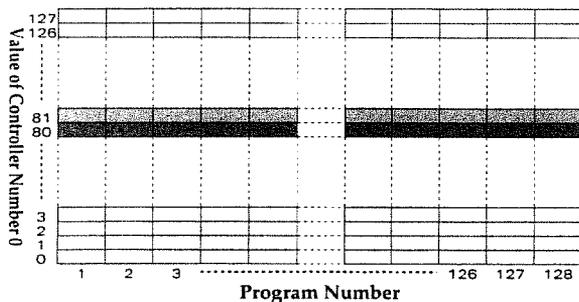
To change a Patch, send MIDI messages from the external device in the sequence shown below.
