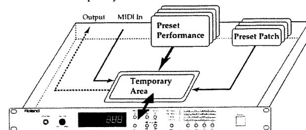
You can change the parameters for Performance or Patch that has been called up into the temporary area. You can also change parameters remotely using an external MIDI device connected to the MIDI in connector.
