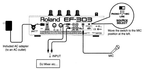
[SOURCE SELECT] switch: In this example we will apply effects to the microphone, so set the switch to "MIC."
