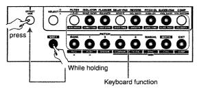
\* Each time you press the [▲] button, the range will be shifted upward by one octave. Each time you press[▼] button.
