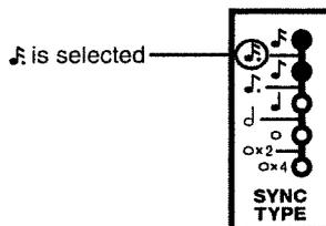
\* [EXIT] + [SYNC TYPE] selects a triplet; the LEDs will be lit in reverse.
