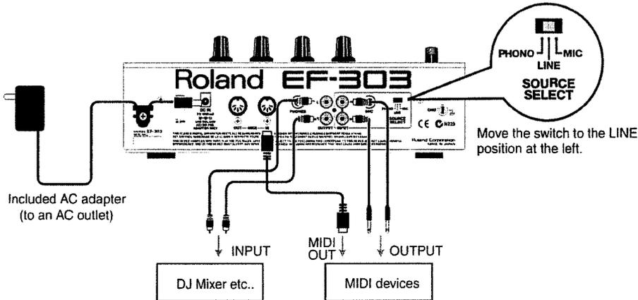
[SOURCE SELECT] switch: Since in this example we will be applying effects to the output signal of the MIDI device, set the switch to "LINE."
