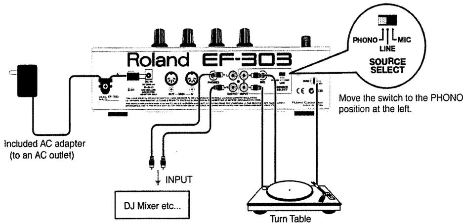
[SOURCE SELECT] switch: In this example we are applying effects to the output signal of a turntable, so set the switch to "PHONO."
