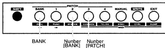
Press the [BANK] button, then press the [2] button. This selects Bank 2. Next, press the [3] button. This selects the "SLICER + PAN" patch of BANK 2 number 3.
