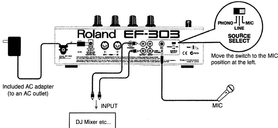
[SOURCE SELECT] switch: In this example we will apply effects to the microphone, so set the switch to "MIC."
