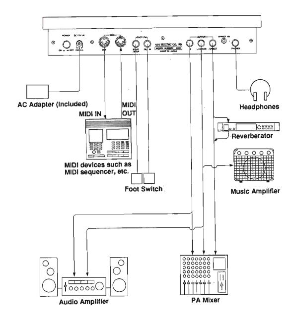
When connecting, always turn OFF the power of your system and XR10. Furthermore, when turning XR10 on or off, keep the volume of a music amp or a mixer at the minimum level never to damage speakers.
