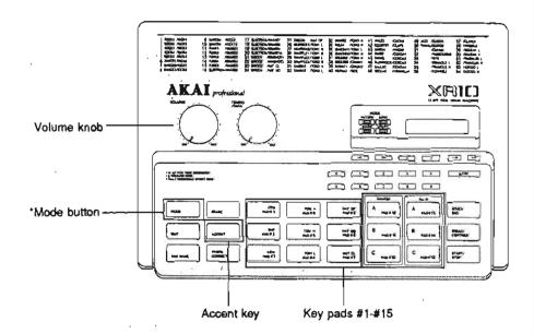
As usual, the sounds will be reproduced by hitting the key pads in any other mode (Pattern, Sound, Utility). When playing the Preset patterns, however, only the sounds assigned to the Key pads #1-#9 can be reproduced. The Key pads #10-#15 will function to select Types of the patterns (Variations A-C, Fill-ins A-C). (For more information refer to p.19).
