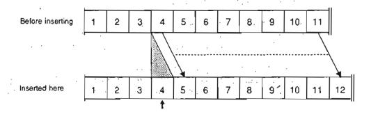
\* The maximum Step sequence entry for one song is 99 steps. Attempting to insert more than 99 steps will not be accepted. The insertion will not be done. The message "OOPS!" shown in the display.
