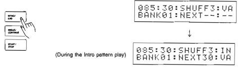
In this case, the last selected Variation Type will be automatically shown in the next pattern field. When the XR10 is turned on, VA (Variation Type A) is automatically selected for the next pattern.
