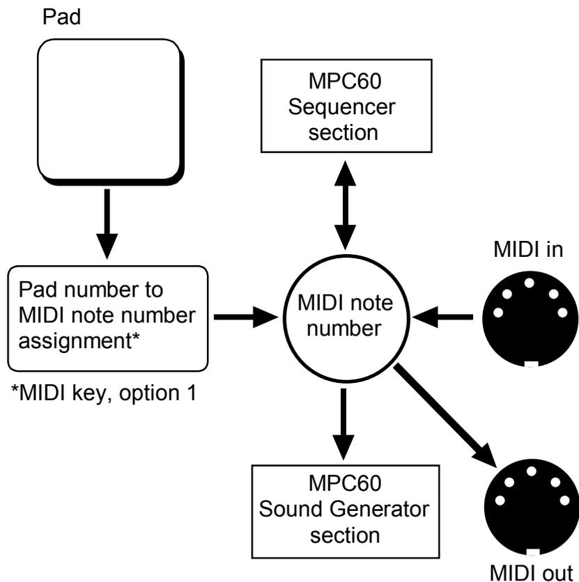
As you can see from the diagram, hitting a pad will generate a pad number, which is then converted into a MIDI note number. This note number can then trigger a sound in the Sound Generator section, be recorded by the Sequencer section, and/or go out the MIDI output. Similarly, note numbers coming in from the MIDI input can trigger a sound and/or be recorded into the sequencer. And note numbers played back by the sequencer can trigger internal sounds and/or go out the MIDI output.
