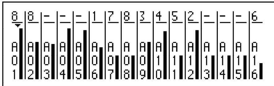
Similar to the Stereo Mix screen, this screen presents a graphic simulation of a multichannel mixer, showing a simulated volume slider and an output assignment for each of the 16 pads in pad bank A (A01–A16). To view other pad banks, press the BANK 2 key.
