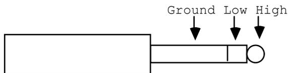
*However, standard mono phone plugs will work fine—the low connection will simply connect to ground*
