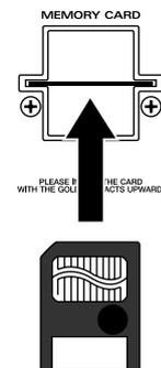
Insert with the surface with the gold connector facing up
