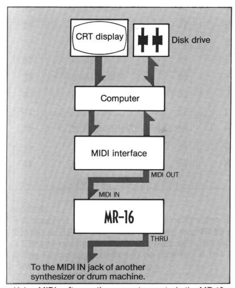
Using MIDI software, the computer controls the MR-16 according to data stored on disk.
