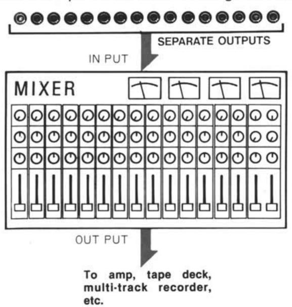
SEPARATE OUTPUT signal level is fixed (not affected by MR-16 volume controls). Use mixing console controls to adjust volume, tone, and position in the stereo image.
