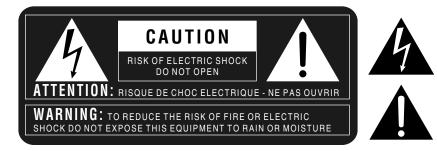
The lightning flash with arrowhead symbol, within an equilateral triangle, is intended to alert the user to the presence of uninsulated idangerous voltageî within the productís enclosure that may be of sufficient magnitude to constitute a risk of electric shock to persons.
